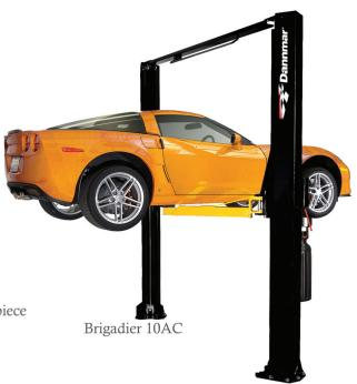
Rotated columns provided added clearance when opening vehicle doors. At the same time, swing-away arms provide a larger drive-thru clearance. Telescoping full-reach arms increase overall arm positioning for lifting a variety of different wheel base vehicles. Overall arm sweep and minimum arm reach are also extended to precisely lift vehicles that have unibody construction, OEM recommended pick-up points and wide and / or narrow wheelbase configurations.
