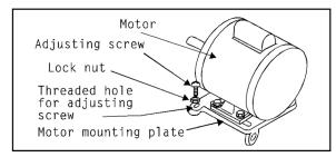
Figure 14: Motor plate adjustment screw
