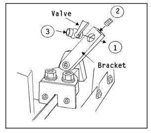
Figure 7: Installing valve in valve bracket
