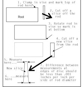
Figure 22: Making a test disc.
