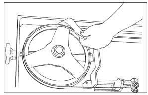
Figure 19: Checking blade tracking
