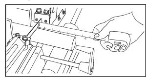
Figure 12: Setting the stock stop cutoff length
