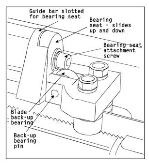
Figure 20: Adjusting back-up bearings
