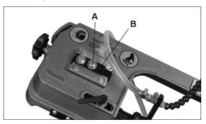
Figure 18: Blade tracking mechanism
