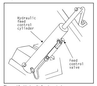
Figure 16: Hydraulic feed control
