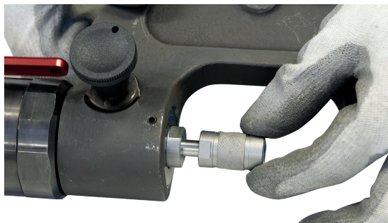
Screw in the included extension to the piston.
