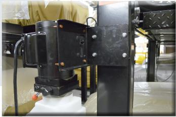
Lift and mount the power unit with the 90° bracket onto the column bracket in either of the positions shown. Tighten the nuts of the 13mm bolts and the installation is complete!
