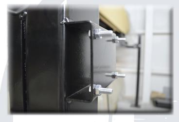
Start with the 13mm bolts originally supplied with your power unit. Install them to the column bracket as shown with one nut tightened.
