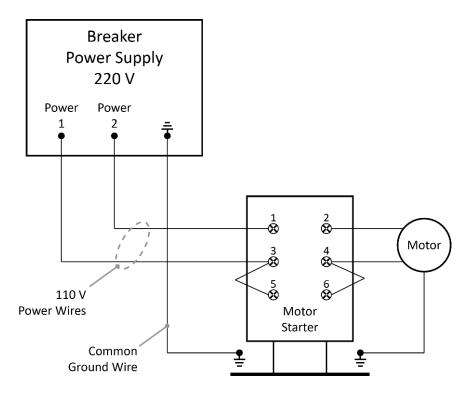
Wiring connections shown, not the physical connections.
