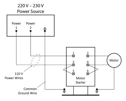
Motor Starter shown in side view for clarity; the Electrical Box is oriented differently. Not necessarily to scale. Not all components shown.
