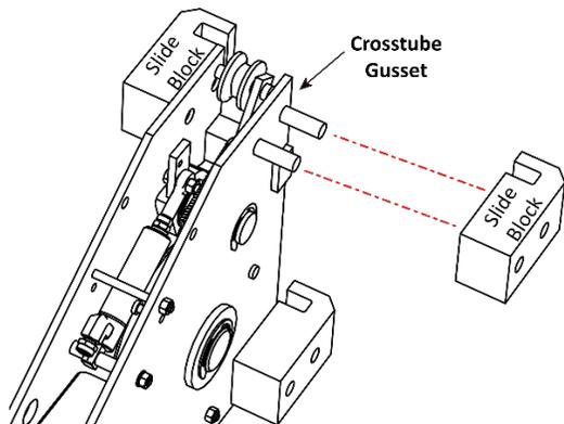
*Top View. Drawing shows how to properly install two Slide Blocks onto the Crosstube Gusset.*
