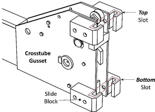
*Front View. Drawing shows the Top and Bottom Slots created by the Slide Blocks. Not all components are shown.*
