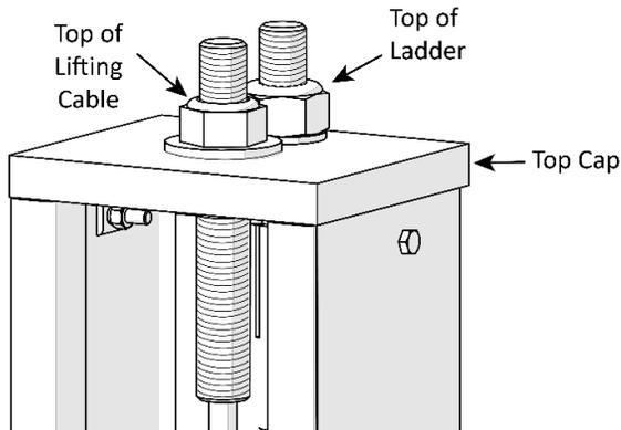
*Drawing shows the Threaded end of the Lifting Cable in position in the Top Cap. View is from the top of the Post. Not all components are shown.*
