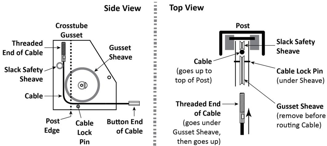
**Important:** When routing a Lifting Cable in its Post, the Cable must go **under** the Gusset Sheave and be on the side of the Slack Safety Sheave. When the Cables are pulled tight, the Cable prevents the Slack Safety from engaging, which is what you want. If the Cable is **not in this exact location**, the Slack Safeties will **not** work correctly.
