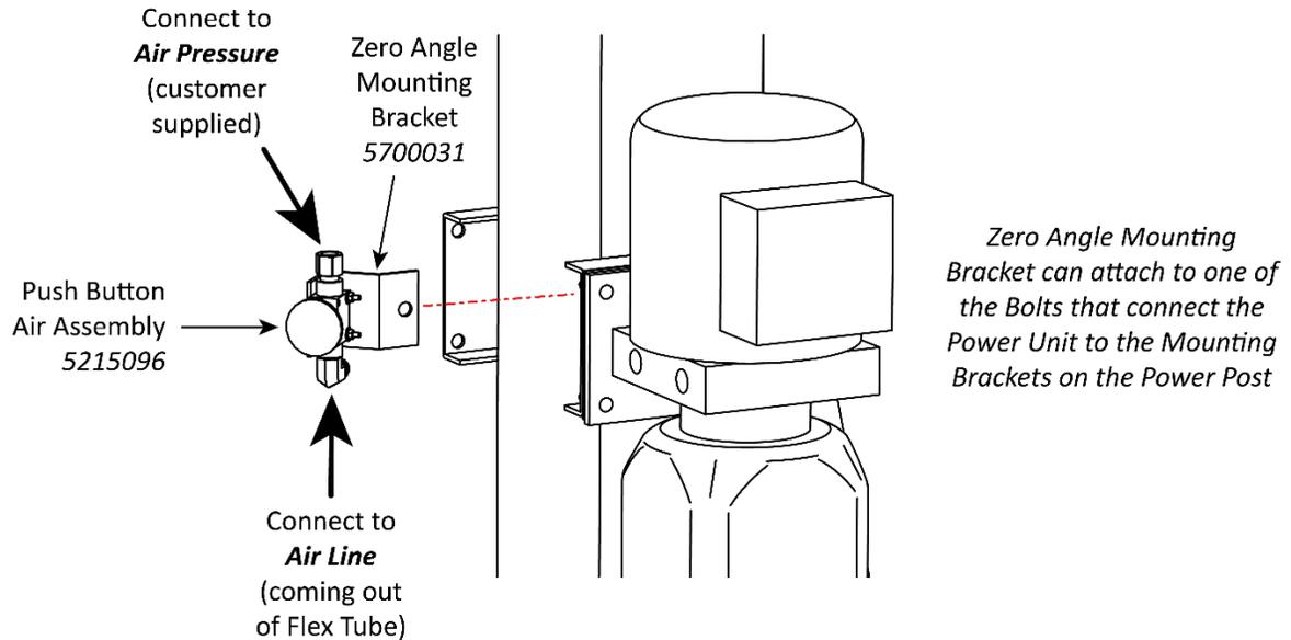
*Drawing shows the Pushbutton Air Valve Assembly and its connections to the Mounting Bracket on the Power Post. Not all components shown. Sample Power Unit shown.*
