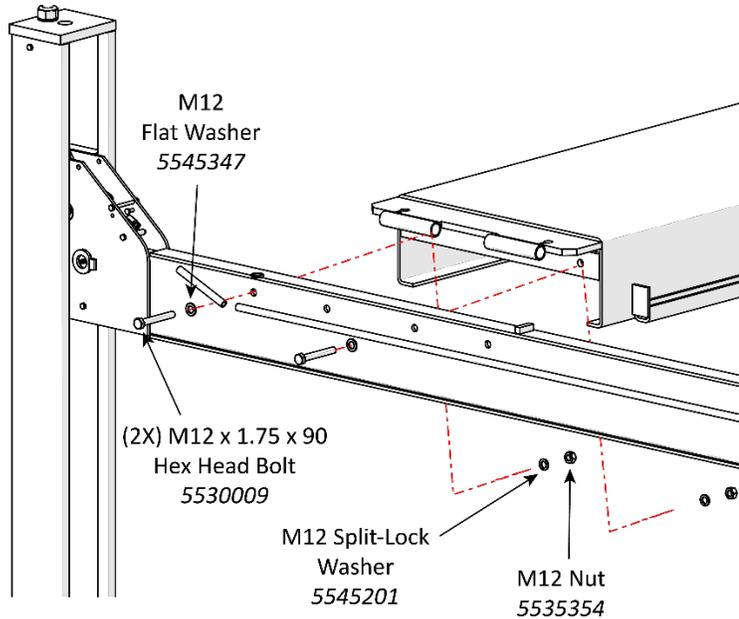
*Drawing shows how to secure the Runways to the Crosstubes.*
