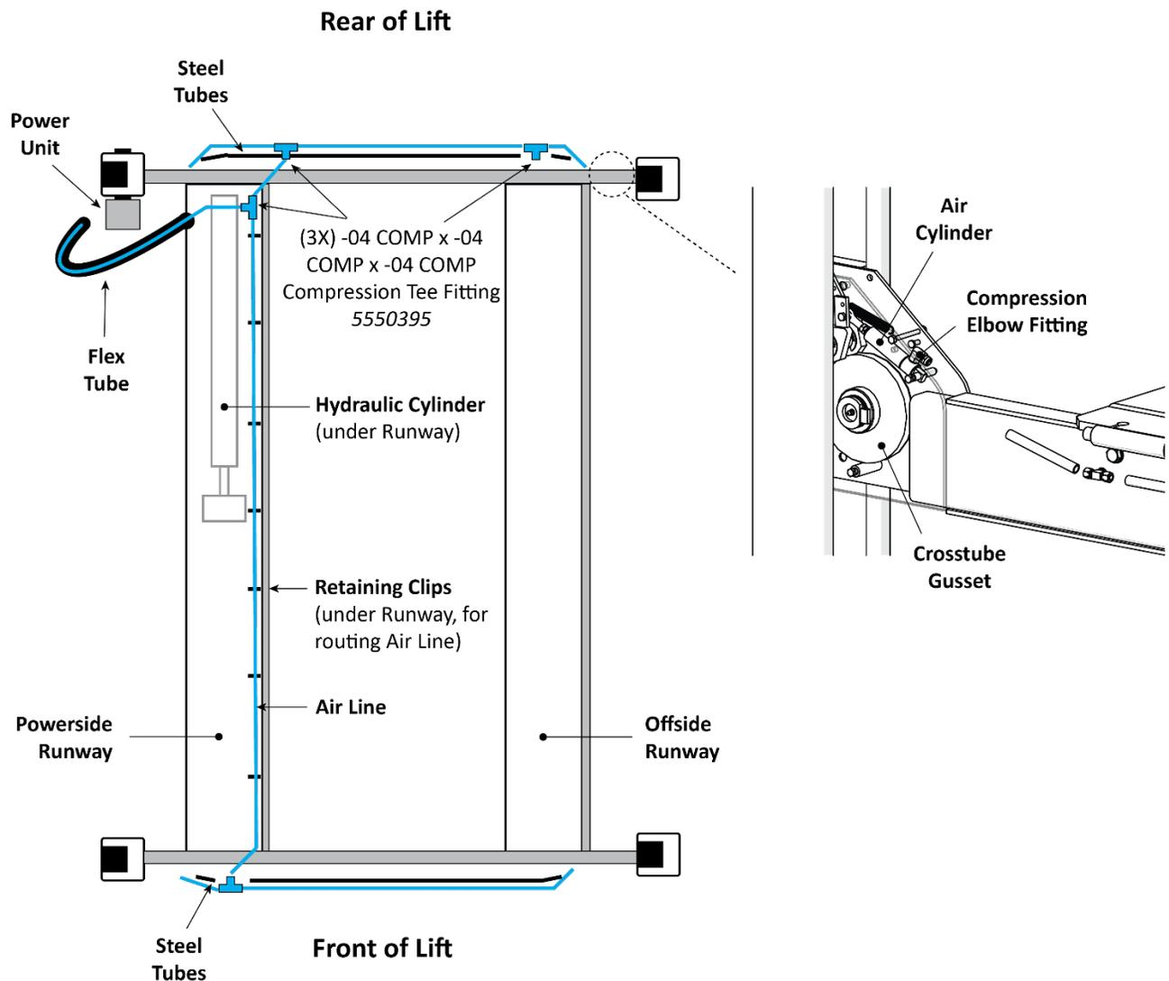
*Air Lines shown outside Steel Tubes for clarity. Drawing not to scale. Some components not shown.*
