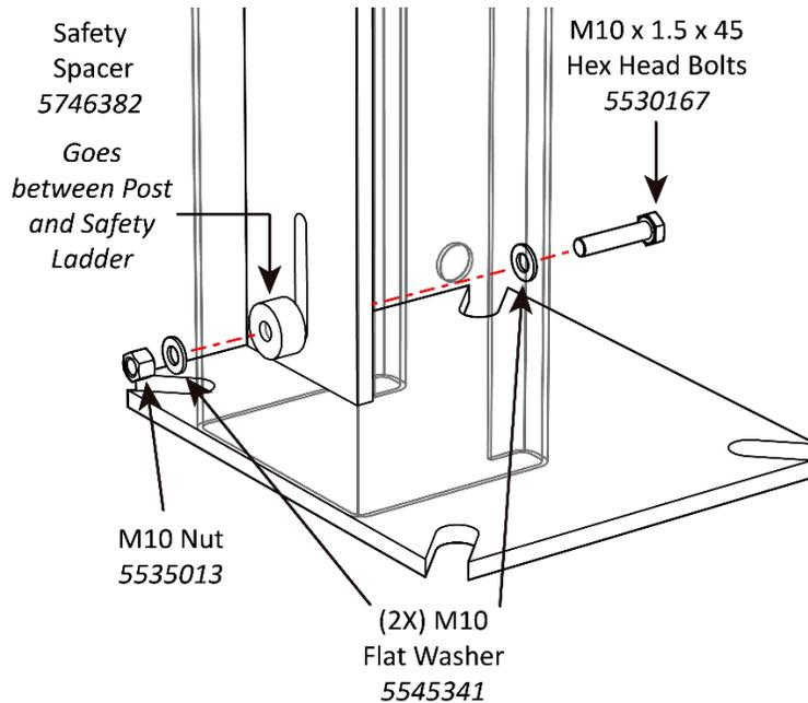
*Drawing shows the connections to make to the bottom of the Post.*
