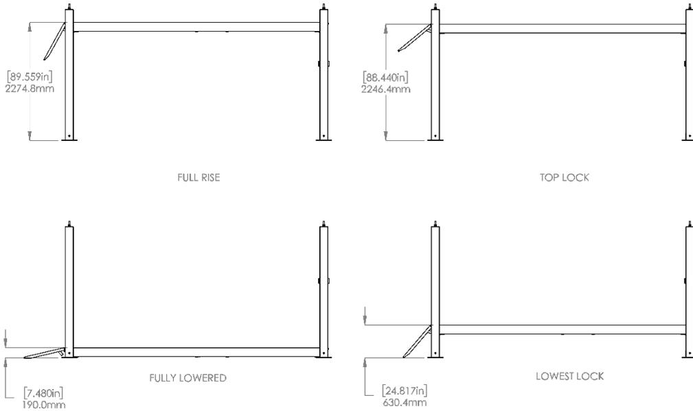
1. DIMENSIONS SHOWN ARE WITH THE LOCK LADDED ADJUSTED ALL THE WAY UP
