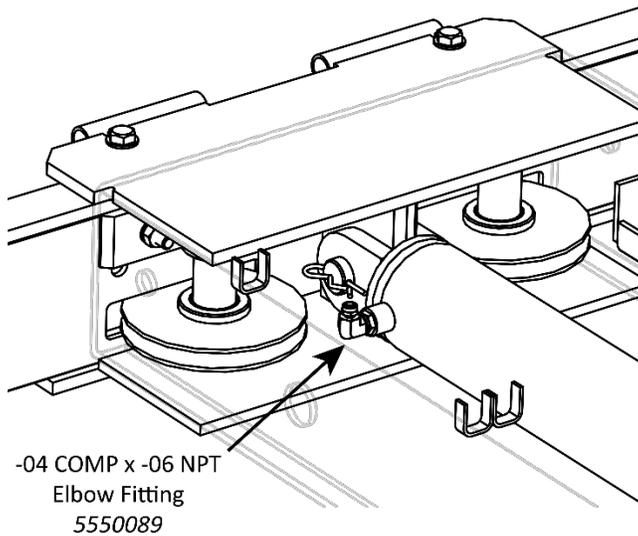
*View is from underneath the Powerside Runway, near Cylinder end. Not all components shown.*
