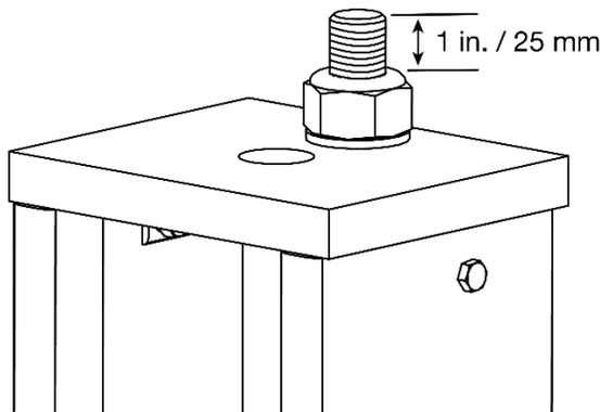
*Drawing shows the threads to leave out above the Top Nut. Adjust as needed.*
