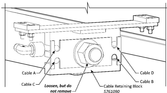
Figure to the right shows the Cable Retaining Block and the Cable positions.
