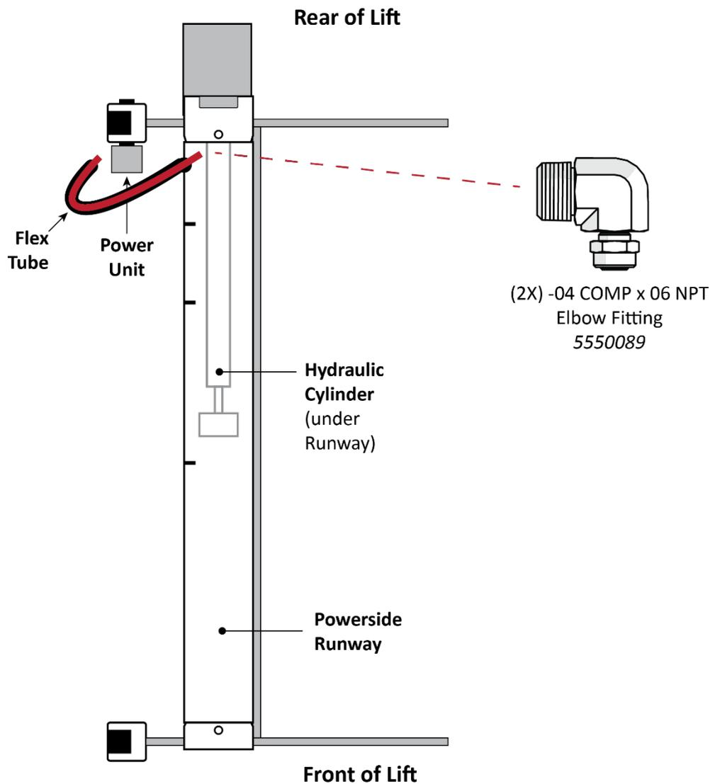
*Drawing shows a top view of the Powerside Runway. Not drawn to scale. Not all components shown.*
