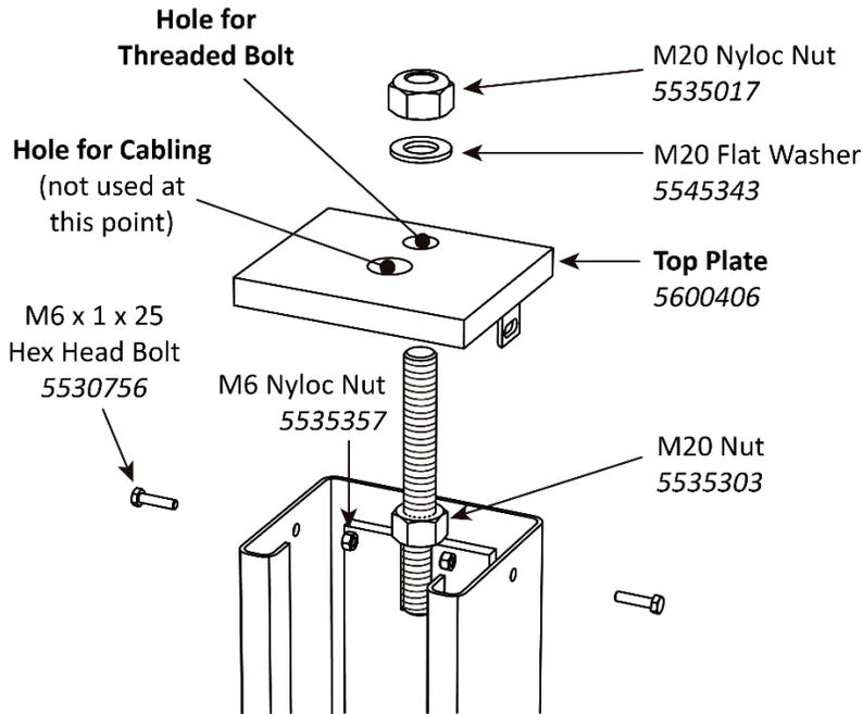
*Drawing shows connections to make to the Top Cap, near the top of the Posts.*
