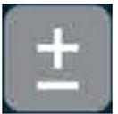
Symbol Key. Press this key to switch the symbol of value in the input area between + (positive) and - (negative).
