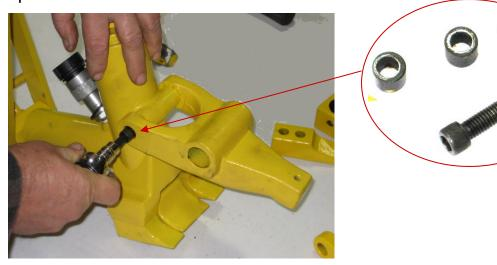
4. Remove the jaw. Using a 3/8 " hex key (allen wrench), remove the Socket Head bolts from the bottom of each foot.
