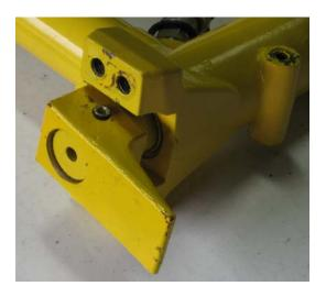
7. Install the 2 larger side feet using the 4 Socket Head bolts.
