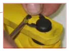
2. Remove the 2 straps, spacer rings, and pivot pin from the jaw. The spacers will **not** be used on the conversion.
