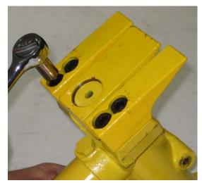
8. Install the new jaw using the 2 Socket Head bolts and spacers.
