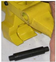
3. Using a 5/16 "hex key (allen wrench), remove both bolts and spacers.
