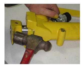
6. Install the new center foot and drive the roll pin in place with a punch and a hammer.
