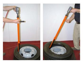
Continue to retract the pulling foot with the impact wrench while bringing the tool towards the wheel center in a pivoting motion until the 1<sup>st</sup> bead is removed. **NOTE:** Do not force or excessively pry with the tool. Allow the natural motion of the pulling foot to remove the tire.
