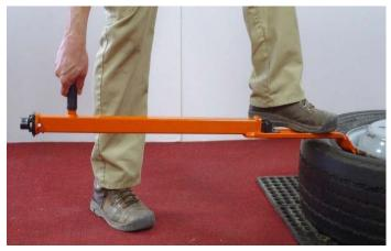
Insert the tool between the rim and tire bead by laying the tool horizontal and using downward pressure with your foot until the heel of the pulling foot is below the plain of the rim.
