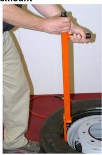
Once inserted between the bead and rim, bring tool to an upright position and ensure that you have a secure hold on the  $2^{nd}$  bead with the pulling foot.
