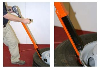
Begin tool engagement by turning the impact wrench in a counter clock wise manner. As the pushing foot begins to meet the rim ensure that the plastic protective angle properly engages the rim edge.
