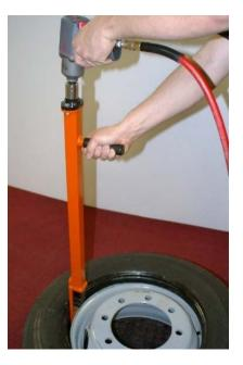
When the first bead is removed turn the impact tool in a clock wise motion too reset the pushing arm.
