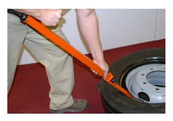
Place tool at an approximately 45 degree angle and insert between 2<sup>nd</sup> tire bead and rim.
