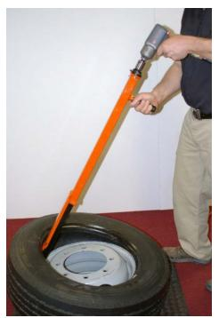
Begin to extend the push foot with an impact wrench in a counter clockwise motion. As the pushing foot begins to meet the rim ensure that the plastic protective angle properly engages the rim edge and allow the natural motion of the tool to rock backwards.
