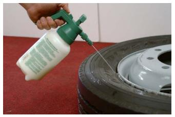
Generously lubricate both sides of the tire before demounting. NOTE: We recommended liquid lubricant to penetrate between rim and tire bead for demounting.
