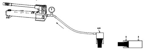
Single-acting cylinders: Position the cylinder so that the plunger is pointed down and the cylinder lower than the pump. Fully extend and retract the cylinder 2 or 3 times. Double-acting cylinders: Lay the cylinder on its side and have the couplers facing up. Fully extend and retract the cylinder 2 or 3 times.
