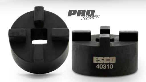
**MODEL 40310 1.8 in. Mack King Pin**Specialty Socket **The ESCO 1.8 in. Mack King Pin Socket** is designed to get the job done safer and easier, while working on Mack trucks. Manufactured for use with 1/2 in. square drive ratchets and breakers bars. Designed to fit the slotted adjusting screw in tapered king pins that are most commonly used on most Mack front axles (12,000 to 20,000 lbs.).
