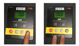
The display screen will show a reading of "**100 PSI**", at this point shut off the air source and calibration is complete.
