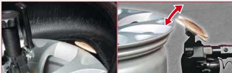
Quick demounting procedure for the second bead, thanks to the **movement of our patented disc** that's particularly suitable for tires with hard walls.
