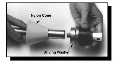
**Step 3** - Place nylon cone over the driving bar. Then select the proper driving washer from the driver range table (see page 2). It is important to use the proper driver washer to prevent damage to the expander assembly. Place the driving washer over the threaded portion of the expander assembly. Screw expander assembly with driving washer into driving bar. (The driver bar extension may be needed for removal of the rear bearings.)
