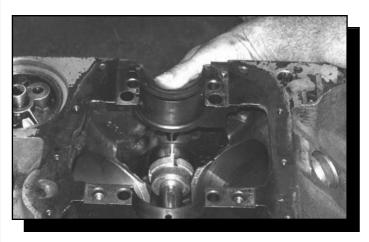
Step 2 - Hold guide cone in place in number one housing and drive bearing. Repeat above steps until all bearings are driven except the number on bearing. To drive the number one bearing, operate from the rear of the engine using the guide cone in the rear housing.
