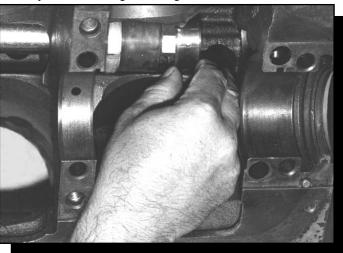
Step 1 - Reduce the expander assembly to its smallest size before installing bearings. Check the separation lines for proper alignment as in figure 2, page 1. Insert tool from the front of the block through the cam bearing housings until immediately in front of the rear bearing housing. Place bearing on expanding driver and tighten until bearing is held firmly.
