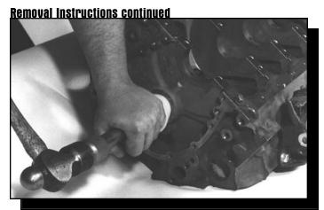
Step 5 - Place nylon cone in first bearing housing and drive bearing out. Loosen driver assembly to relieve pressure and pull tool back through the next bearing to be driven. Repeat above steps
