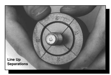
**Step 2** - Check to insure that separation lines between segments of expanding driver line up with separation lines on the expander assembly as above.
