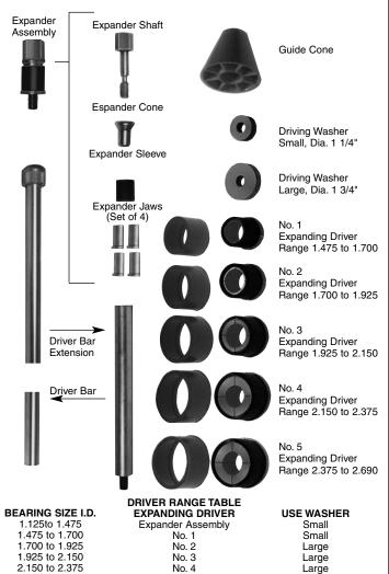
**NOTE:** This tool has two sets of rubber sleeves supplied with it for the expanding drivers. The brown sleeves are used when driving thin wall bearings (.065). The black sleeves should be used when driving thick wall bearing (.090). See instructions below for changing the sleeves.
