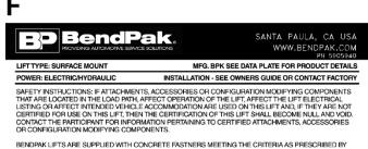
BENDPAK LIFTS ARE SUPPLIED WITH CONCRETE FASTNERS MEETING THE CRITERIA AS PRESCRIBED BY ASTM £488 - 96(2003). LIFT BUYERS ARE RESPONSIBLE FOR ANY SPECIAL REGIONAL STRUCTURAL AND/OR SEISMIC ANCHORING REQUIREMENTS SPECIRED BY ANY OTHER AGENCIES AND/OR CODES SUCH AS THE UNIFORM BUILDING CODE (UBC) AND/OR INTERNATIONAL BUILDING CODE (IBC).
