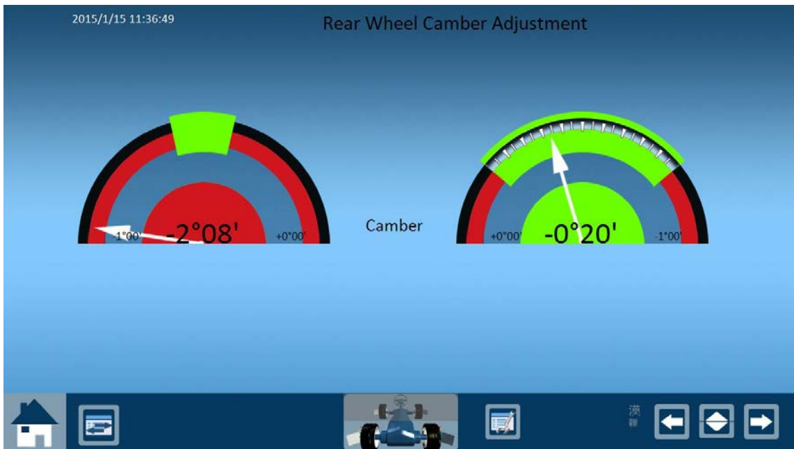
Individual adjustment of rear wheel Camber
