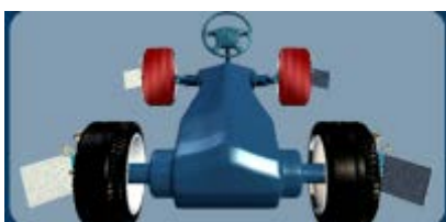
Front targets both blocked
