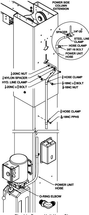
Fig. 14 - Power Unit Hose Clamps
