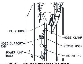
Fig. 16 – Power Side Hose Routing
