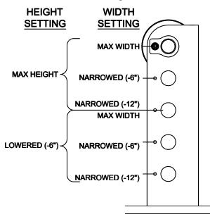
Fig. 2 – Sheave Position in Lower Bracket
