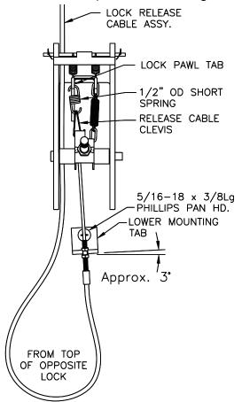
Fig. 18b-Lock Release – Idler Side
