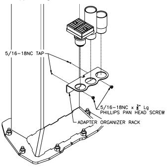
Fig 22-Adapter Rack Installation
