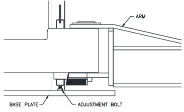
Fig. 21-Bolt Adjustment
