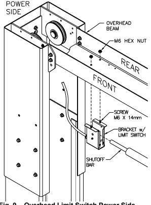
Fig. 9 – Overhead Limit Switch Power Side
