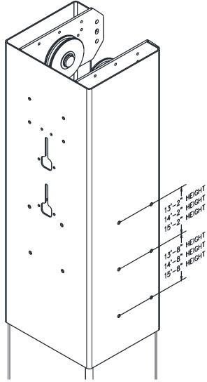
Fig. 5 – Column Extension Assembly
