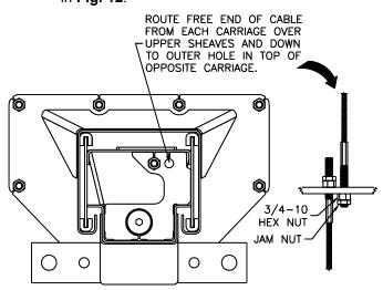
Fig. 12 – Cable Attachment at the Carriage
