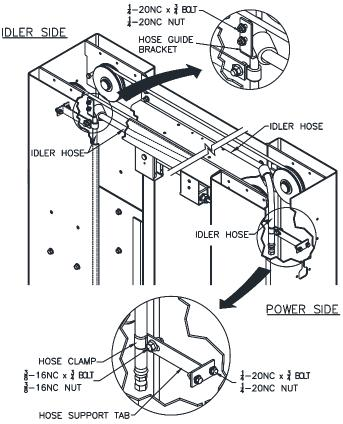
Fig. 13 – Idler Hose Routing & Hose Brackets
