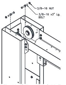
Fig. 11 – Column Ext. Cable Trapping 33) Mount synchronizer cables to carriages as shown in Fig. 12.
