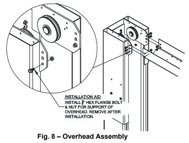
28) Check idler column shimming. Use additional shims (*see Fig. 7*) to remove any gaps that may have been created while installing overhead beam. Tighten anchor bolts and re-check column for plumb. Torque to 150 foot-pounds.
