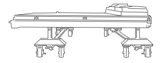
4. Fully lower battery onto the extension pad assembly. Ensure all pins are properly located to secure the battery to the dollies. Detach the overhead lifting apparatus. NOTE: Use caution while moving battery as weight of the battery may impede maneuverability and require additional time/distance to bring battery to stop.
