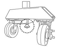
3. Tighten the knurled adjustment bolt that secures each outrigger base assembly to the tie bar to dollies bearing the full battery weight. NOTE: Failure to tighten adjustment bolts prior to the dollies bearing the battery weight may result in unsafe shifting/detaching of the outrigger base assembly.
