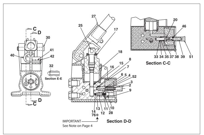
Figure 3. Sections B-B, C-C and D-D
