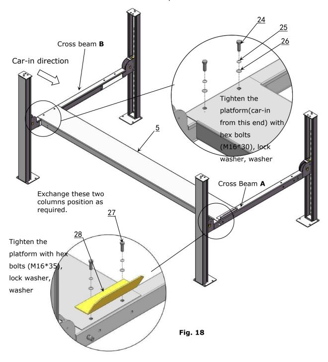
G. Install offside platform and limit block, then install the bolts for the platform strengthen plate, check the plumbness of columns with level and adjusting with the shims (See Fig. 19).
