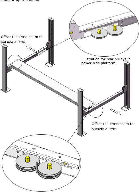
Illustration for front pulleys in power-side platform
