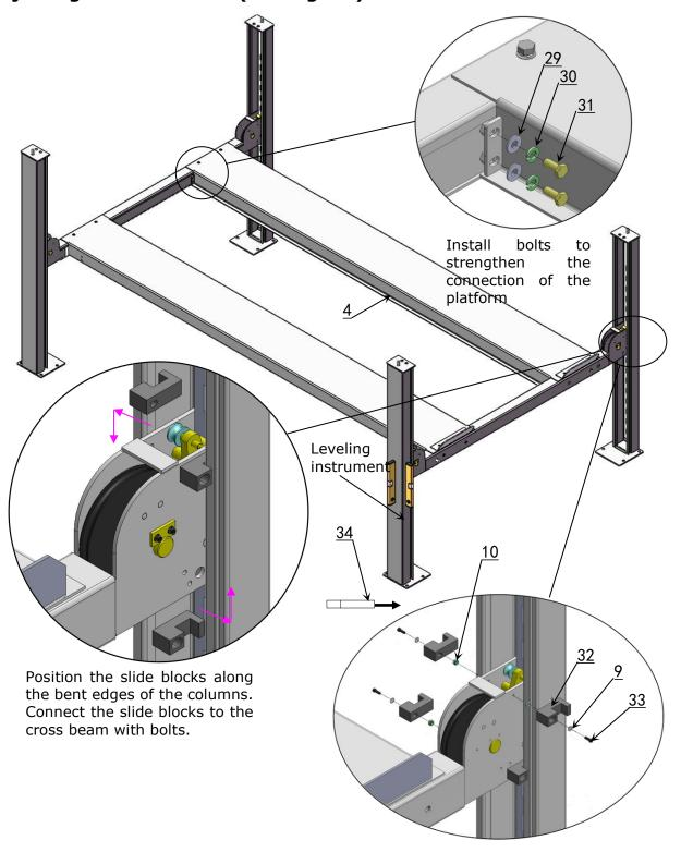
**Note: DO NOT** completely tighten the limit slide blocks. Loosen 1/4 lap after tightening.
