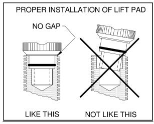
Fig. 1: Proper installation of lift pad
