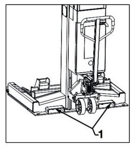
Fig. 15: Forklift pocket locations 1 Forklift pockets
