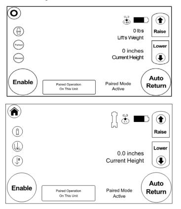
5. All the buttons shown function in the same way as described in Section 8.5 and 8.6. The vehicle can be raised or lowered as needed to place stands and support the vehicle. The distance the vehicle can be raised or lowered is limited while in single or paired mode.
