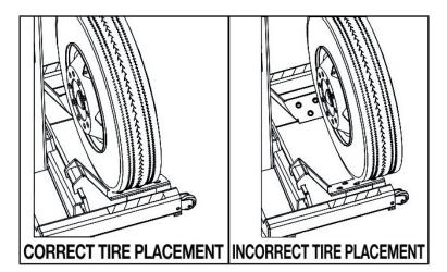
Fig. 6: Position lift table tube against tire
