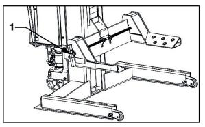
Fig. 18: Wide model carriage width adjustment 1 Carriage adjustment screw
