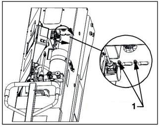
Fig. 20: Down stop grease fittings 1 Vent screw
