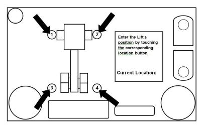
Fig. 8: Enter lift position in relation to vehicle
