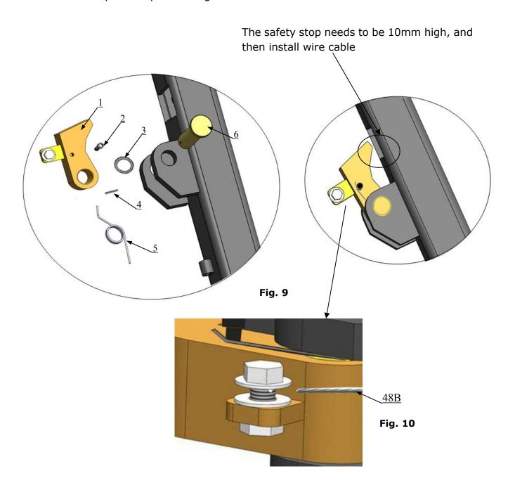
Put the small wire rope into the hole on the screw and then tighten
