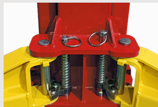
• Lifting arms lock automatic release device, high strength gear rack, more stable and reliable.
