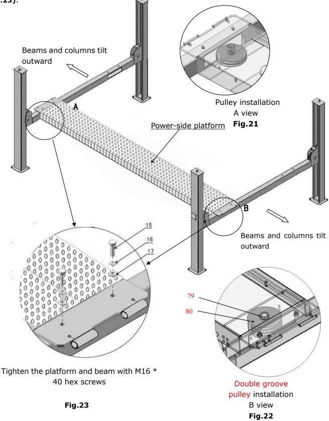
I. Assembly offside platform and slider block, (See Fig. 24) check the plumbness of columns with level, adjusting with the shims if not, and then tighten the anchor bolts (See Fig. 25).
