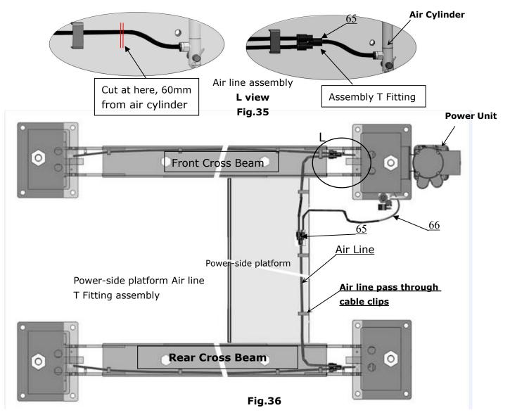
Connecting air solenoid valve using / \phi8\*\phi6 black air line
