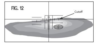
INTERNAL SCREEN: VOL BEAM PATTERN
