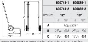
\*Handle height of cart is adjustable to 355/8", 385/8", 411/2" or 441/2". Eight 5/16" (8mm) diameter mounting holes.
