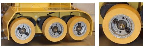
The roller wheels have specially formulated rubber tires (left) that grip well without marring the wood. Each wheel can be easily replaced individually. Each also has its own grease fitting (right) to keep maintenance simple.
