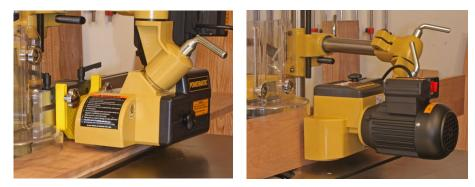
The articulated arms and universal joints allow using the Powermatic PF3-JR feeder to move stock flat on the table (left) or on edge at the shaper (right) for molding or face cuts.
