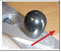
STEP 8 - Unlocked position to remove the retaining unit.
