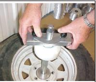
STEP 7 - Locked position when holding the wheel.
