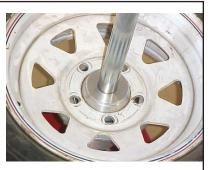
STEP 6 - Place the retaining unit over the shaft while holding out the two knobs. Turn approximately 1/4 turn to lock.
