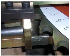
Anti-springback lever disengaged
