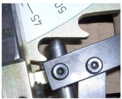
Anti-springback lever engaged
