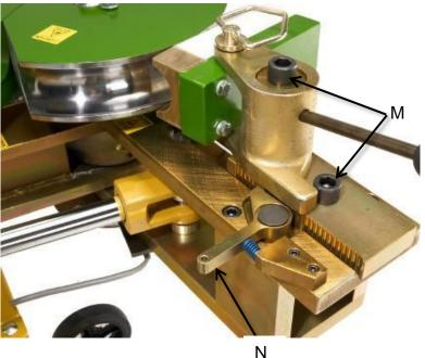
IMPORTANT: THE RATCHET WILL FAIL IF THE BOLTS ARE NOT TIGHTENED PROPERLY.
