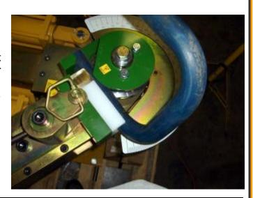
IMPORTANT: Orienting your material in this fashion will cause damage to your tooling and machine!! DO NOT pull bent material into the counter die! Make sure you have enough straight material on the draw side of the material to create your bend.
