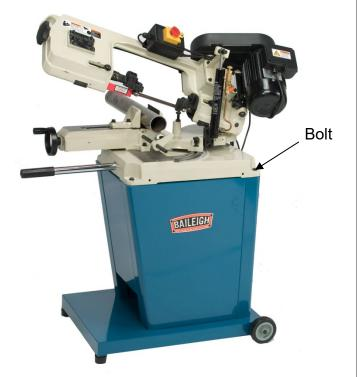
4. Attach the stop bar to the base as shown and tighten setscrew. (Can also be mounted on left hand side.)
