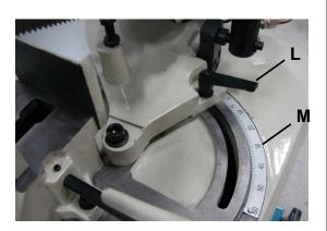
CAUTION: Check that the saw blade clears all parts of the vise assembly before cutting. The blade can strike parts of the assembly (especially during miter cuts) if not properly adjusted.
