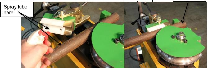
3. With the die head at home or "0" position, insert material past the hook arm aligning the "0" mark on the die with where the bend will start on the material.
