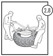
This step is best performed with the cooperation of two personnel. Standing at opposing ends of the adjusting rods pick up the discharge assembly using proper lifting techniques and position the assembly directly over the wheel.
