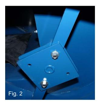
If a smaller cullet is preferred additional Breaker Bars are available. Each unit comes with two Breaker Bars and can operate with up to four.
