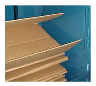
5. Do not load cardboard with loose flaps facing up. Face them down. Cycle the unit several times if necessary to compress contents. Check the completion of bale by looking through Sight Window in upper door. Maximum compression is 2400 psi on gauge.
