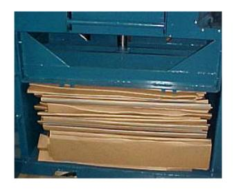
6. STOP unit by pushing red Emergency Stop button after the ram passes by the sight window making a complete and full compression. Remove Safety Lock T and open lower door.
