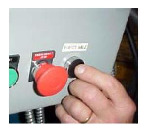
14. Press and hold EJECT Bale button. This raises the cable hook in back, pulling on the cable, lifting the bale out.
