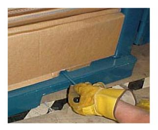
8. Locate White Decal marker and plunge wire from the front of the unit through to the back of the unit. (This operation is done twice.) Go to back of unit and remove wire from Plunger eyelet.
