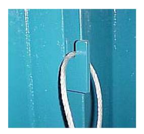
13. See step 3. Take wire from hook and place loop end of Cable on this Lift Hook located in the back center of the unit.
