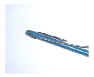
7. Each bale requires two pieces of wire to wrap around and hold bale tight. With one wire thread roughly 3 inches of it through eyelet of supplied Wire Plunger.
