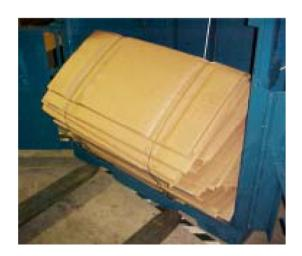
15. Bale being Ejected by the cable looped on lifting hook. When bale is removed place a piece of cardboard in bottom of crushing chamber – prepping for next bale to be made.
