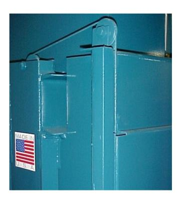
A safe-guard on the TC-720 is the Locking Door feature (see left.) Pull the handle towards you to open.
