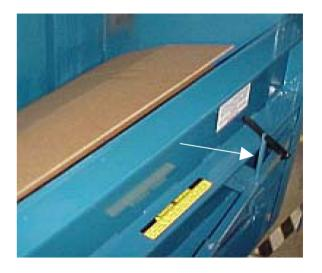
4. Load chamber with cardboard. Note the "Safety Lock T" pin in place with lower unit door closed.
