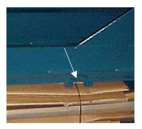
10. From the front of unit guide the plunger rod through to the back of the unit (see arrow.)
