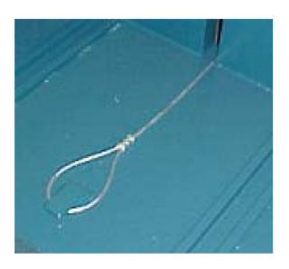
2. Cycle the unit and open bale chamber. Open lower door. Loop one end of supplied cable on inner tab in bottom as shown.
