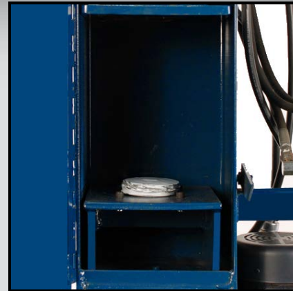
TC-15 Detail Crushing Chamber
