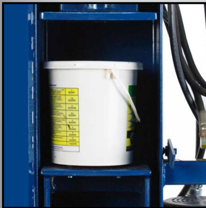
TC-15 Detail Crushing Chamber
