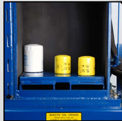
TC-16 Detail Crushing Chamber
