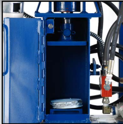
TC-6 Detail Crushing Chamber
