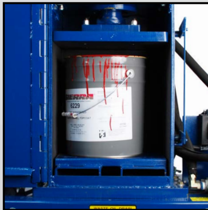
TC-16 Detail Crushing Chamber
