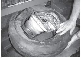
Slide the wheel and tire out of the TC-300 chamber. NOTE: The wheel and tire can be taken out of either side of the machine
