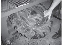
Slide the wheel and tire out of the TC-300 chamber. NOTE: The wheel & tire can be taken out of either side of the machine
