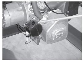
This photo illustrates the Oil filter location on the engine. Replace filter every 6 months for smooth engine operation
