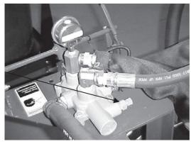
If the valve "kicks out" on the arms return stroke, the detent will have to be tightened slightly. Loosen lock nut as shown. Tighten outer nut 1/4 turn and tighten lock nut. Continue to crush. If it "kicks out" again, readjust it another 1/4 turn.
