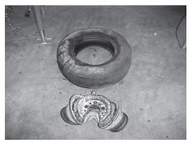
This photo illustrates the wheel crushed and separated from the tire.
