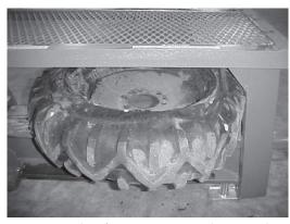
Position tire to the front against the crushing frame as shown.
