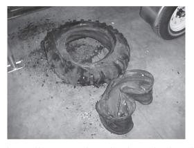
This photo illustrates the wheel crushed and separated from the tire.
