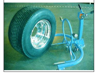
Align the Tweel handler into position under tire.
