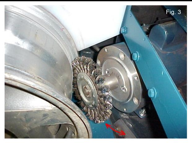
Make a visual inspection of the rim to determine if flange and bead seat area are complete. When that side of the rim is finished crank motor position away from contacting the rim and turn unit OFF.
