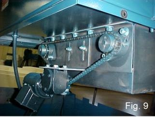
Grease all four bearing zerks as needed. (Too much grease collects dirt.)
