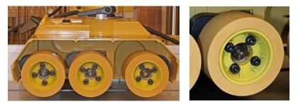
Each of the wheels (left) is mounted on its own suspension arm to help keep it in firm contact with the material. Each wheel is easily replaced individually and has its own grease fitting at its center, (right)
