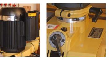
The PF-31 motor (left) is pure heavy-duty, starting with the cast iron case with integral cooling fins. The switch (lower right) on the feeder body selects the high and low speed ranges.
