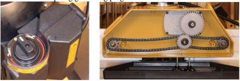
The switch on the motor (left) controls forward or reverse feed directions. The gears can be reversed to produce a second high/low feed rate.
