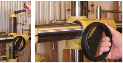
The support column (left) and arm (right are made from heavy-walled steel tubing. Both have easy to use adjustments that make setting the PF-33 up for use simple.
