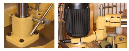
The column assembly gives the POWERMATIC PF-31 Stock Feeder 9-3/4" of vertical movement, controlled by a top-mounted crank that drives a lead screw. There is a full 18" of horizontal
