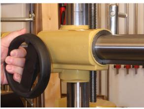
The vertical adjustment (left) uses a top-mounted crank operating a lead screw. The horizontal arm (right) is adjusted using the handwheel that engages a gear drive. Both adjustments have tool-free locking levers.
