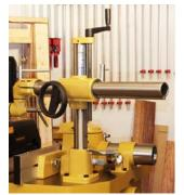
The support column and arm assembly is made from tough cast iron and steel for maximum rigidity.
