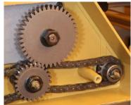
The motor power is sent to the wheels via a slip-free chain and gear (left) drive system.
