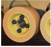
All four wheels (left) are mounted on individual suspension arms to insure a consistent, firm grip on the wood. Each wheel has a grease fitting at its center. The wheels are easy to change and can be replaced individually if needed.
