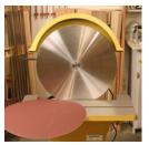
The spacious cast iron table tilts 30-degrees up and 45-degrees down for easy bevel sanding of virtually any angle. The table also can be raised and lowered for maximum versatility and for changing abrasive discs.
