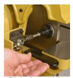
This hand-operated disc brake lets the operator stop the heavy platen in seconds and do it safely.
