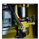
Five spindle speeds (3,000 to 10,000 rpm) with speed indicator. Fast speed change and tensioning device and big 71/2HP motor.
