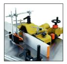
Fence assembly includes hold downs with full coverage guard, dust collection, adjustable fence halves and dual digital readout positioning with micrometer adjustments.
