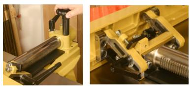
The fence has a gear drive (left) that makes positioning it on the table easy and accurate. The mechanism that controls bevel settings (right) is all cast iron with adjustable stops and easy to use locks.
