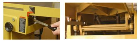
Both tables have easy to use handles (left) and locking knobs. The dual spring assist (right) makes these massive cast iron tables "feel" much lighter than they really are when making height adjustments.
