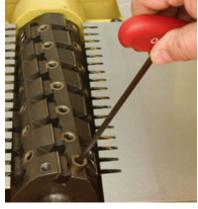
The helical insert head is specially designed to drastically reduce the upward pressure most wide helical heads put on the wood.
