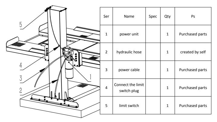
Note: Only fresh and clean hydraulic oil is allowed, and 46# hydraulic oil is recommended; do not fill the oil barrel completely for the first refueling, the hydraulic oil volume can meet the lifting platform to the highest level; Suggestion: replace the hydraulic oil with new hydraulic oil 6 months after the first use, and then replace it once a year;
