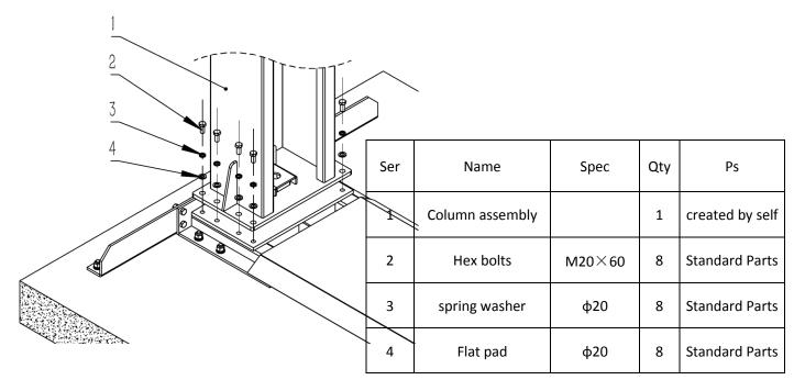
3.8 - Attachment yoke installation (as shown in the picture)
