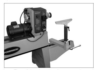
Figure 6-7: outboard turning accessories
