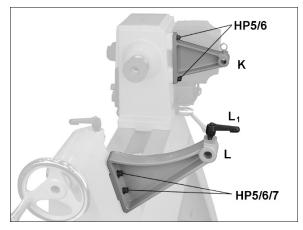
Figure 6-3: installing brackets
