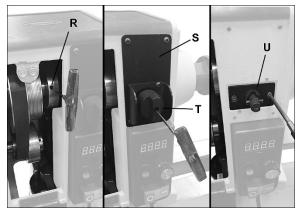
Figure 8-10: sensor and spindle lock collars
