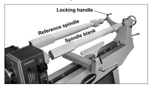
Figure 8-7: comparator (shown with optional 20" bed extension)
