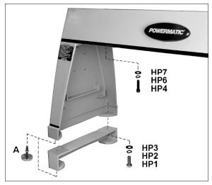
Figure 6-1: installing legs and riser blocks
