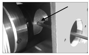
Figure 8-11: loosen spindle lock collar
