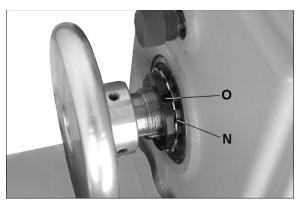
Figure 8-12: correcting spindle play
