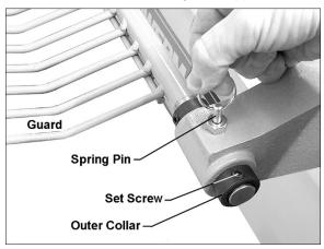
Figure 6-4: installing optional guard
