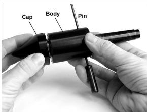
Figure 8-3: live center cap removal
