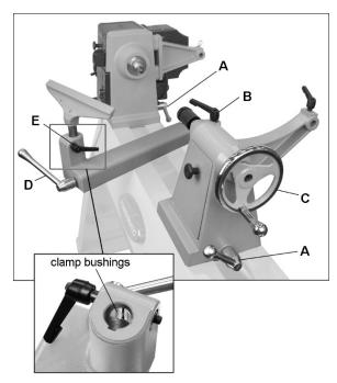
Figure 8-1: headstock, tailstock, tool support
