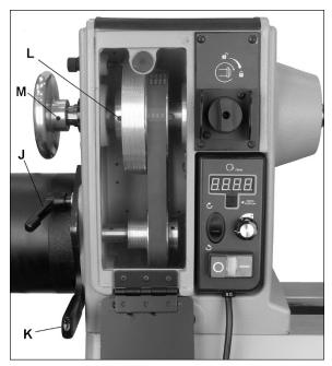
Figure 8-9: sheave/belt alignment
