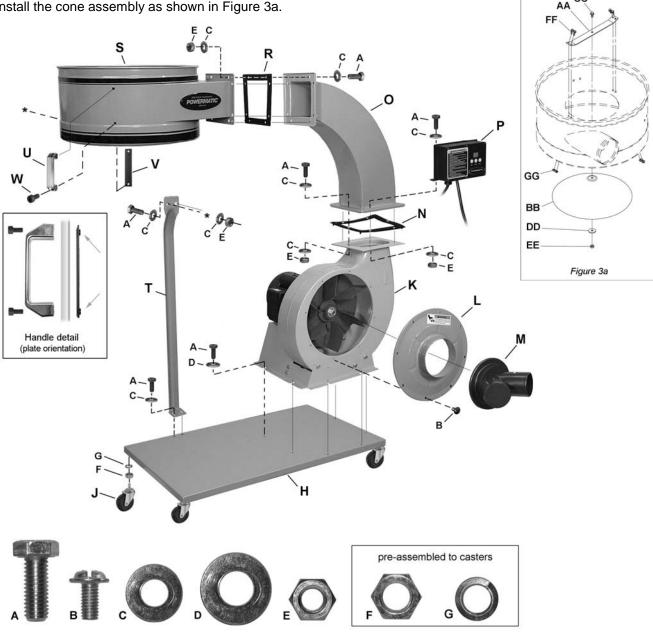
Figure 3: Assembly and hardware identification
