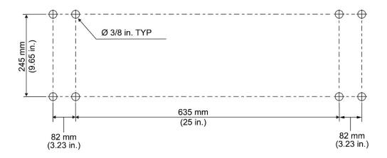
Figure 4-1: mounting pattern for workbench
