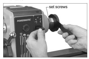
Figure 8-7: installing/removing faceplate
