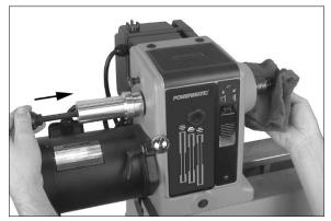
Figure 8-5: removing center from headstock
