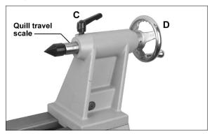
Figure 8-6: installing center in tailstock
