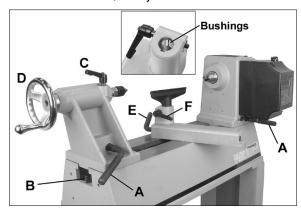
Figure 8-1: headstock, tailstock, tool support
