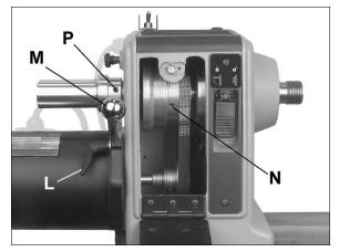
Figure 8-9: sheave/belt alignment
